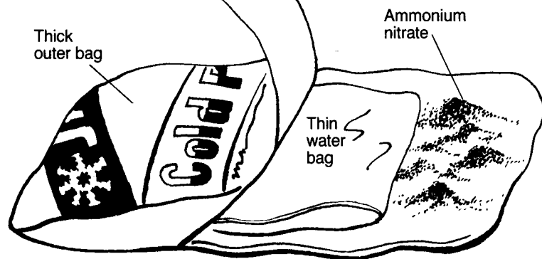
Figure 1. Jack Frost brand instant cold pack. The ammonium nitrate crystals and a plastic bag of water are contained inside a heavier plastic bag. Punching the pack bursts open the inner bag, allowing the water and ammonium nitrate to mix.
